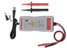
UT-P33 Differential probe 120MHz 14kV
