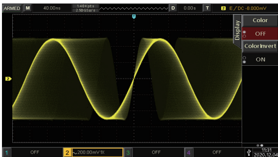
● Up to 200,000wms/s waveform capture rate, improving the ability of capturing the random and low probability events, observing the signal jitters and glitches clearly
