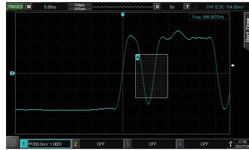
● The area trigger can be used in combination with the existing basic trigger, advanced trigger and protocol trigger to complete the capture of various occasional and complex characteristic signals.
