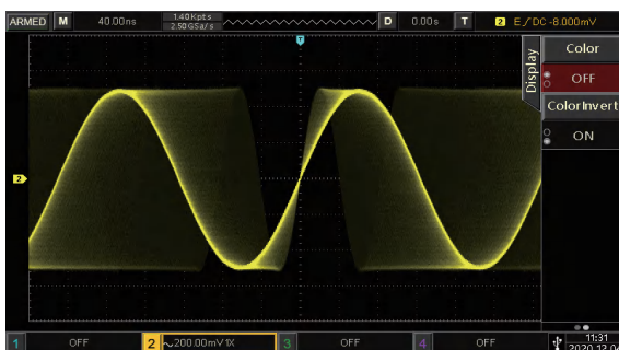
● Up to 200,000wfms/s waveform capture rate, improving the ability of capturing the random and low probability events, observing the signal jitters and glitches clearly
