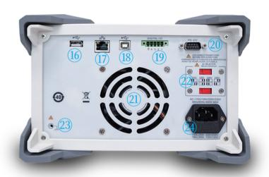
①LCD display ②Function key ③Digital keyboard ④Rotary encoder ⑤Shift key ⑥Channel selection and output control ⑦Keyboard lock ⑧Preset key ⑨System settings ⑩Home key ⑪CH3 quick selection ⑫Operation menu ⑬Power switch ⑭CH4 output ⑮Output channel and indicator ⑯USB HOST ⑰LAN ⑱USB device ⑲Digital IO ⑳RS232 ㉑Fan ㉑Input source selection ㉑Protected GND ㉑AC socket
