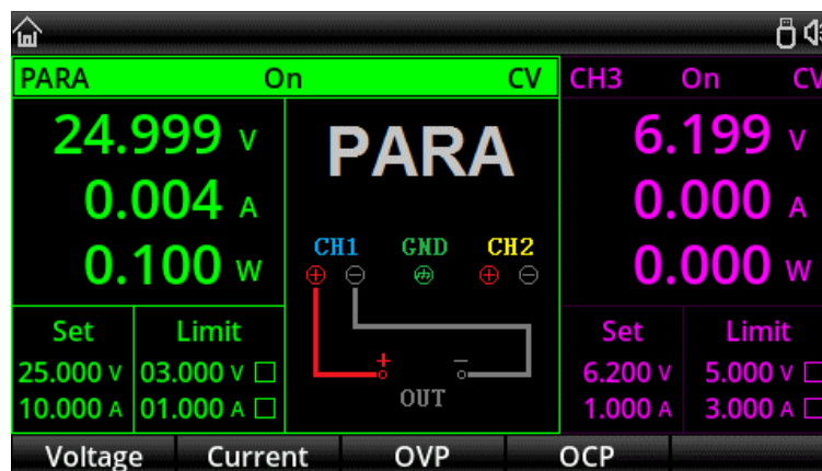
Parallel Connection Setting Interface
