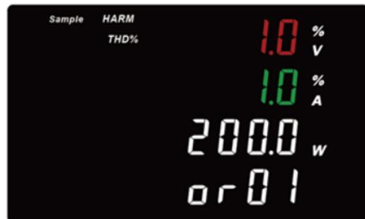
Press "THD/%" key to select "THD%" mode to enter the relative value of total harmonic wave measurement. Press "▲, ▼" to select the absolute value of sub-harmonic wave.
