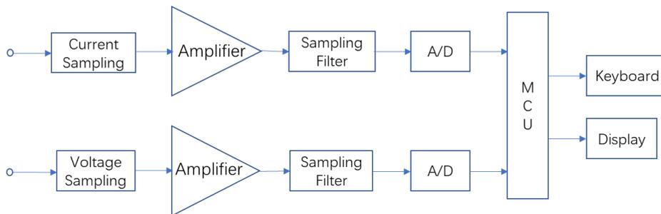
As shown in the figure, the instrument consists of an analog part and a digital part. The analog part is mainly composed of sensors, multi-grade programmable amplifiers, sampling filters, A/D and other circuits. The digital part consists of microcomputer data memory, keyboard and display.
