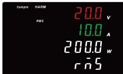
Press "THD/%" key to select "THD%" mode to enter the relative value of total harmonic wave measurement. Press "▲, ▼" to select the relative value of sub-harmonic wave.
