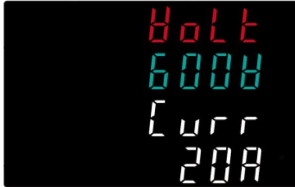
Window 2: the current voltage range, "600V", "300V", "150V", "75V".
