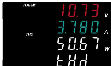
Window 4 displays "tHD" or "or01"~"or50". "tHD" represents the total harmonic distortion; "or01"~"or50" represents the currently selected harmonic times. The display item of window 4 can switch by **【↑】** or **【↓】**.
