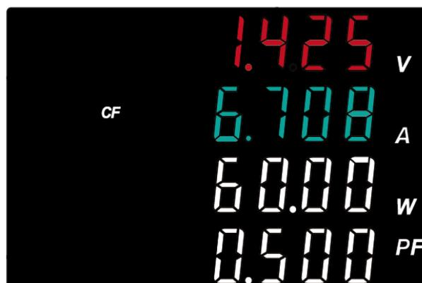
Window 1: the measured value of voltage crest factor, no unit. The measured value of voltage crest factor= Voltage crest value/ TRMS Voltage. When no voltage signal is input, it displays "-----".
