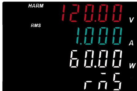
Window 1: the total RMS voltage (operation value) of 1~50 times, the unit is V.
