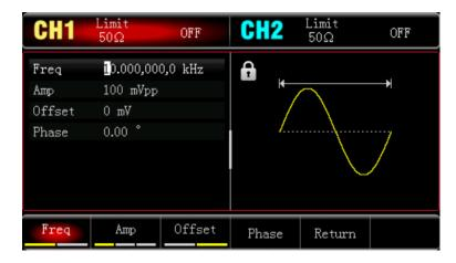
Press Freq soft key to set the frequency, use numerical keyboard to input 900 and then select the unit of parameter to Hz;
