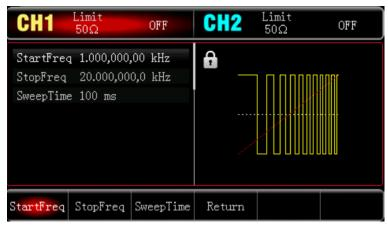
Press Start or Stop soft key, use numerical keyboard to input 1 and then select the unit of parameter to kHz. The default start frequency is 1 kHz.
