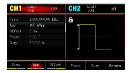
Press Freq key to set the frequency, use numerical keyboard to input 1 and then select the unit of parameter to kHz;
