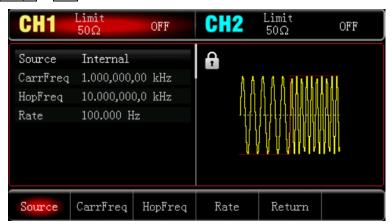
2) Set Hopping Frequency and Modulation Rate
