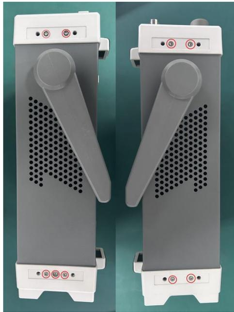
2. Gently remove the front panel, as shown in the figure below.
