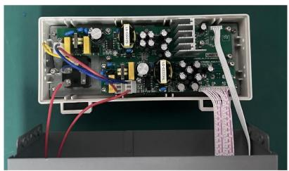
2. Remove the power module; use a T10 Torque screwdriver to remove the 6 screws and the wiring harness, as shown in the figure below:
