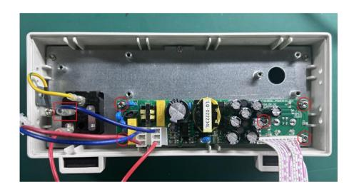
4. Remove the rear panel; use a T10 Torque screwdriver to remove the 6 screws and the grounding wire, as shown in the figure below:
