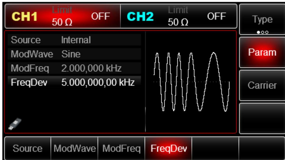
The shape of FM modulation waveform checked through oscilloscope is shown as following:
