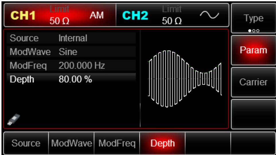
The shape of AM modulation waveform checked through oscilloscope is shown as following:
