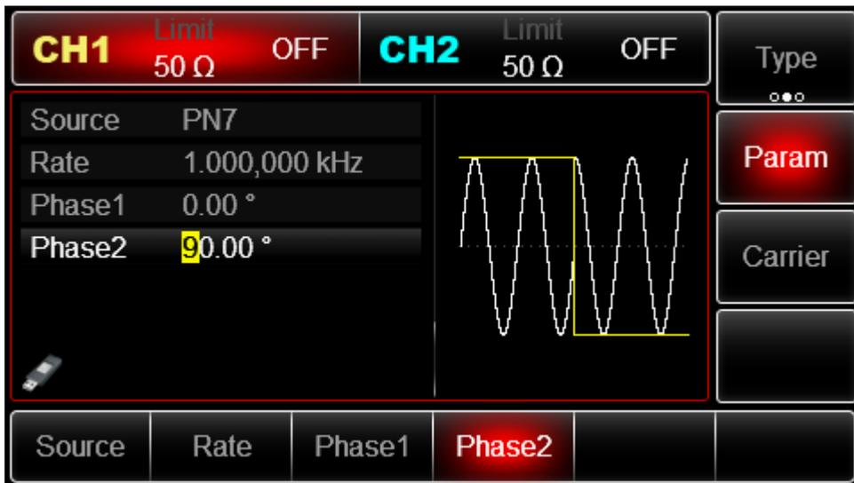
Check the shape of BPSK modulation waveform through oscilloscope, which is shown in the figure below:
