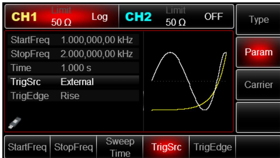
Figure 3 - 38 Select external trigger source
