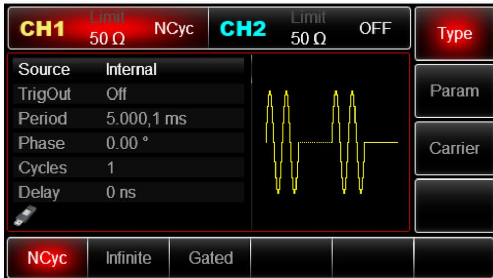
Figure 3 - 55 Set pulse train parameters
