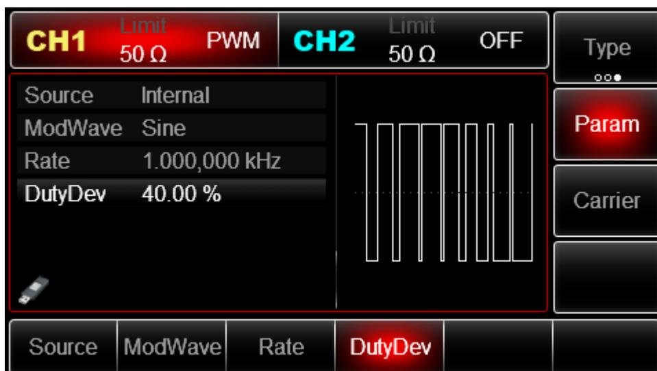
Check the shape of PWM modulation waveform through oscilloscope, which is shown in the figure below:
