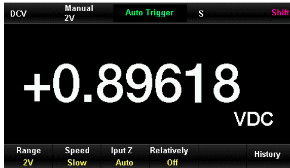
Figure 2-4 Interface of DC voltage measurement
