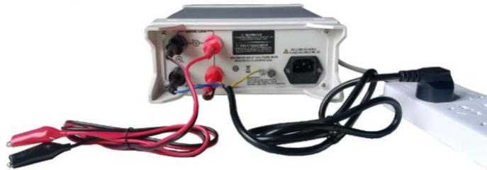
Warning: Before connect with circuit, please make sure the power is cut off to prevent from electric shock.
