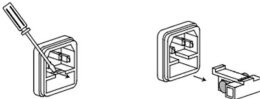
If the fuse was burned out, please replace the same specification fuse with the instrument. The specification fuse with the instrument, see the following table.
