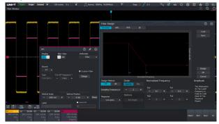
The user-defined advanced filter designer can be directly configured on the oscilloscope.
