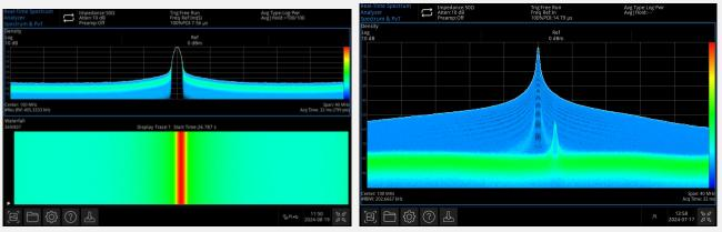
Use combined display with density spectrograms for continuous spectral display, visualizing the frequency occurrence of signals and capturing small signals in the presence of larger ones
