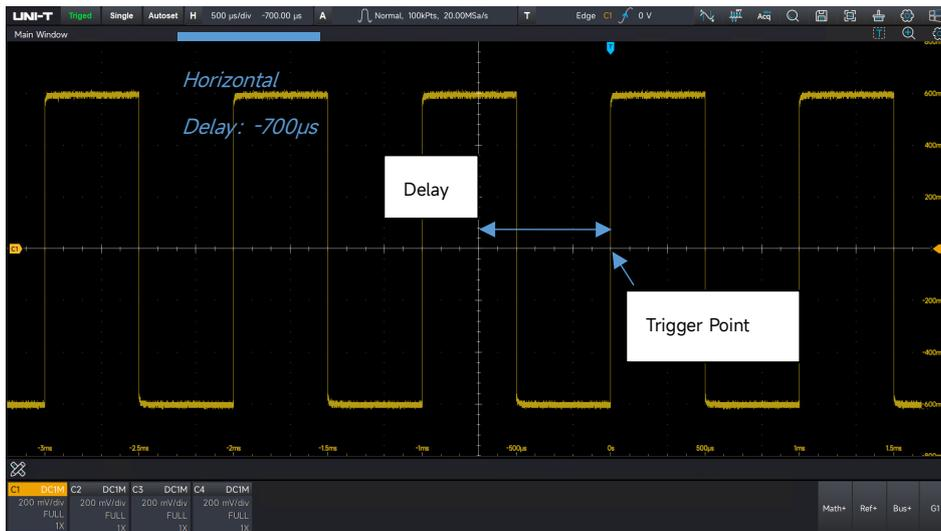
When changing the horizontal delay, the waveform will move left or right along with the trigger point.
