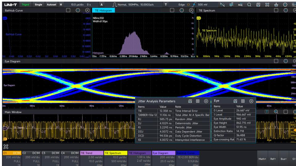
TIE (Time Interval Error) represents the timing error of a signal relative to the reference clock. In high-speed digital systems, TIE refers to jitter, and in this oscilloscope, it specifically refers to the  $TIE_{peak-peak}$ . The measured signal's edge is compared with the ideal edge established by the clock recovery, and all signal intervals are measured based on the ideal data rate.
