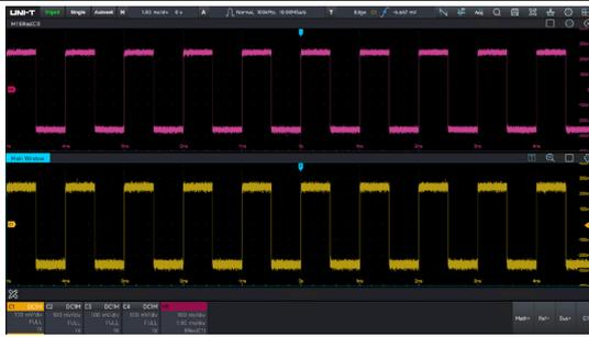
Unprocessed waveform: noise 70mV
