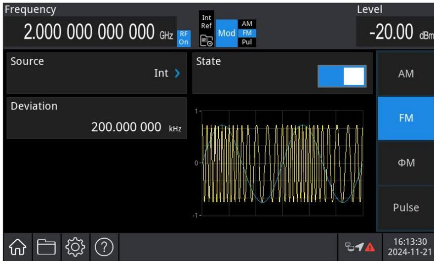
View the FM modulation waveform on a spectrum analyzer, as shown in the following figure.
