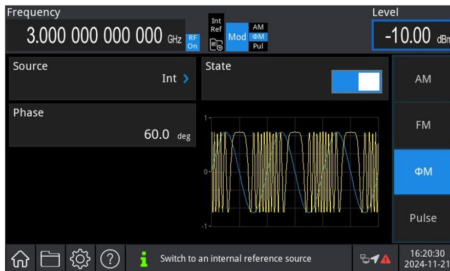
View the ΦM modulation waveform on a spectrum analyzer, as shown in the following figure.
