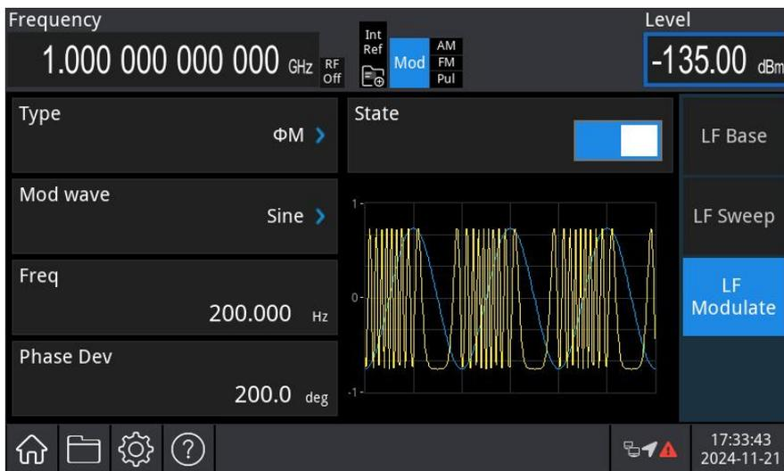
View the  $\Phi M$  modulation waveform on an oscilloscope, as shown in the following figure.
