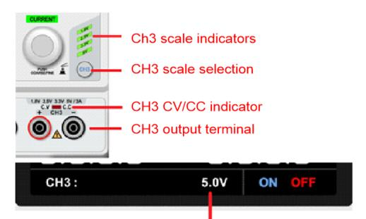
The CH3 selected voltage scale is lit on LCD
