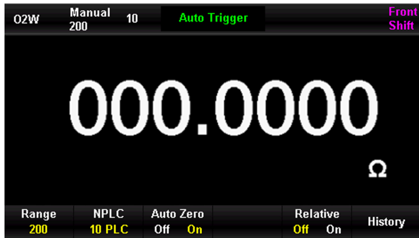
Figure 4-3 Reading of Test Wire Short-circuit
