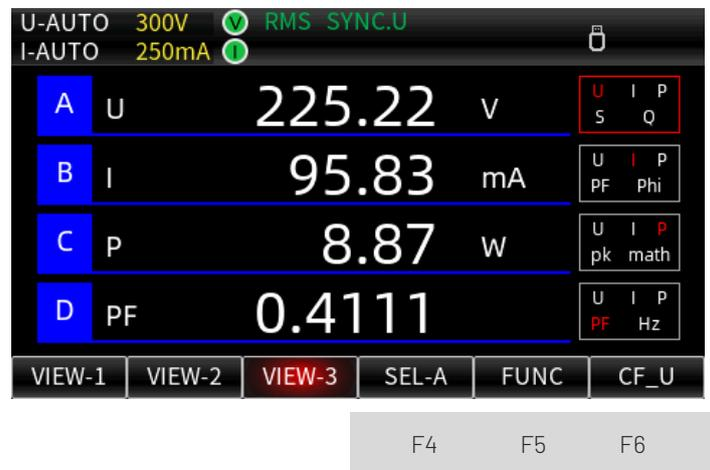
When selecting the VIEW-3 display style, the measurement window will be increased by three positions of F4, F5, F6 corresponding to the function indication. For the sake of simplicity, respectively, use F4, F5, and F6 to describe its function in this subsection.
