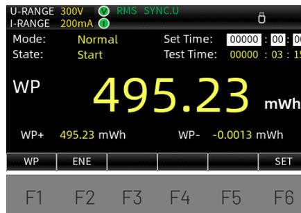
1. In the integration interface, press the "F1" key to switch to the power integration WP or the current integration q.
