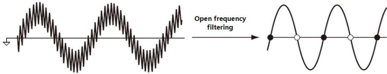
Note: The frequency filter is not inserted in the measurement circuit of voltage and current, and even if the frequency filter is enabled, the measured values contain high frequency components.
