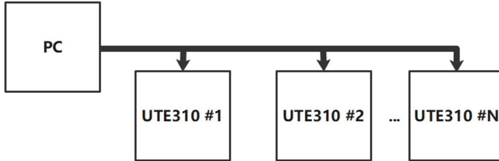
In normal condition, PC has no GPIB interface, the user can connect through the GPIB to USB converter card, as shown in the following figure.
