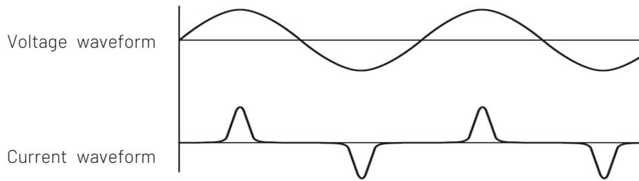
If the measurement object is a switching power supply, the voltage and current waveforms are shown in the figure, and from the waveforms, it can be seen that the voltage waveform has less distortion compared to the current signal, so the voltage signal should be set as a synchronous source at this time.
