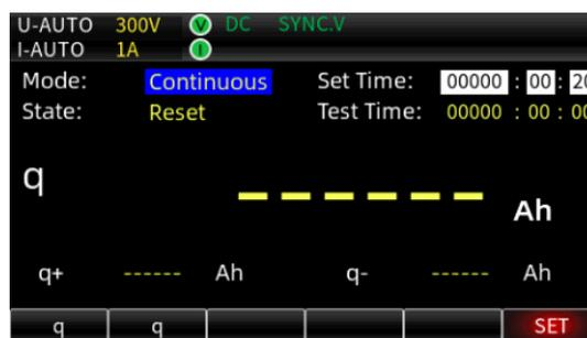
2. Select the integration mode "Continuous" or "Normal" by pressing the [◀] or [▶] key.
