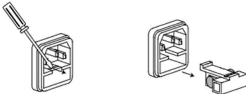
If the fuse was burned out, please replace the same specification fuse with the instrument.
