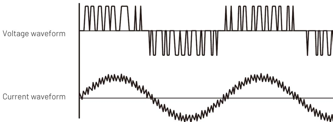
If the measurement object is a converter, the voltage and current waveforms are shown in the figure, and from the waveforms, it can be seen that the current waveform has less distortion compared to the voltage signal, so the current signal should be set as a synchronous source at this time.
