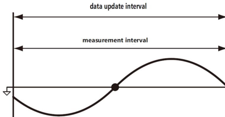
The UTE300 series digital power meter calculates the measurement data by averaging the sampled data within the measurement interval. The period of the input signal is detected from the voltage and current signals, and the user can set either the voltage signal or the current signal as the synchronization source.
