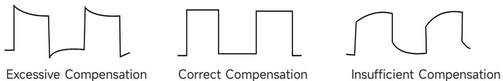
Figure 2 Compensating Calibration of Probe
