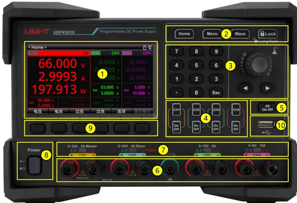
Figure 2-3 UDP4303S Front Panel
