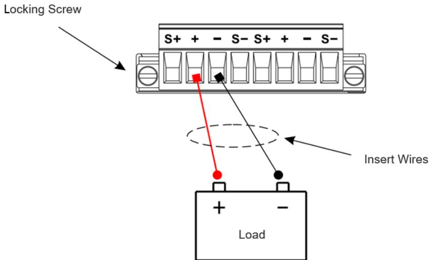
Figure 2-8 Rear Outputs Connections
