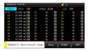
Or users could press [MULT ZERO] key, and use the Numeric Keypad to enter channel number to do the zero clearing. (channels need to be short-circuited before zero clearing start.)
