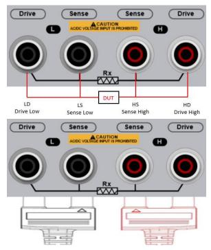
Multi-channel scanning test terminal shown as below. D+/D+ represents Drive High and Drive Low; S+/S- represents Sense High and Sense Low.
