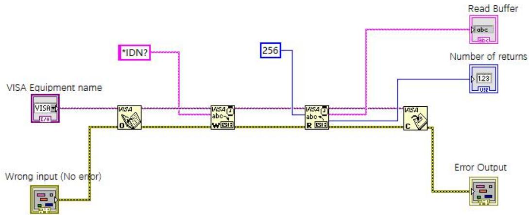
5. Communication with the device via TCP/IP is similar with UBTM, it need to set VISA write and read function to synchronous I/O, set LabVIEW to asynchronous IO by default. Right click on the node and select "Synchronous I/O Mode>>Synchronous" from shortcut menu to enable synchronous writing or reading of data, as shown in the following figure.
