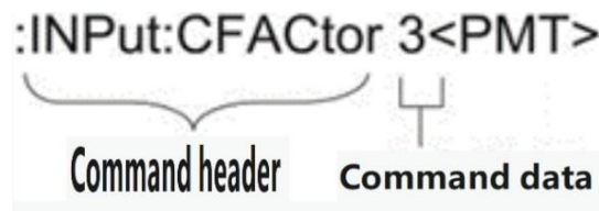
Figure 2.4 Example of command header and command data
