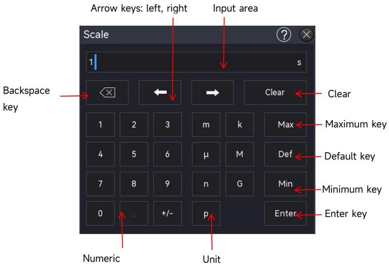
After entering all the values and selecting the desired units, the numeric keypad will automatically close, completing the parameter setting. Additionally, the user can manually close the numeric keypad by clicking the confirm key, in which case the unit will default to the preset unit. On the numeric keypad, the user can also perform the following operations:
