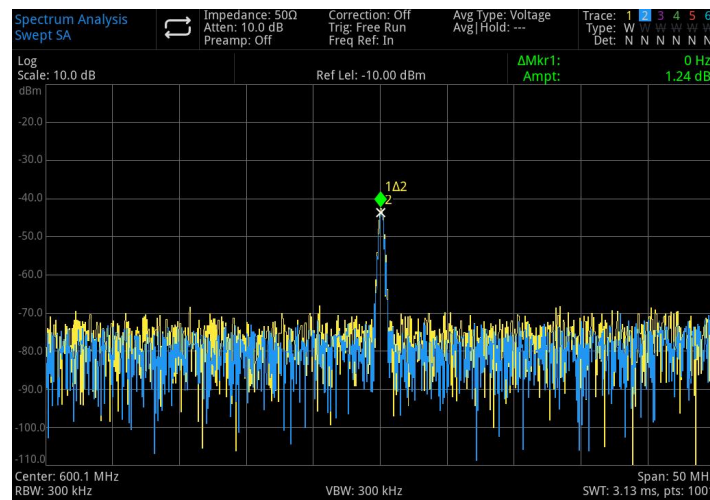
Figure 3-17 Component of Harmonic Distortion
