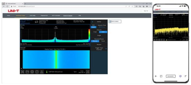
Supports SCPI remote control, remote viewing, and control of exported trace data, as well as other operations. It enables online browsing and use and supports access from both PCs and mobile phones.
