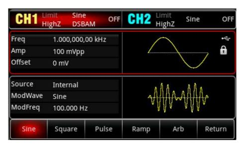
Press the softkey Freq, and then use the numerical keyboard to enter 2 kHz.
