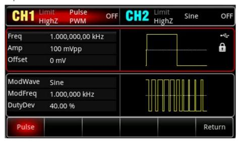
Press the softkey Freq to set the frequency, use the numerical keyboard to enter 10 and then select the unit of parameter to kHz.
