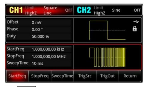
Press the softkey StartFreq to set the start frequency, use the numerical keyboard to input 1 and then select the unit of parameter to kHz. The default is 1 kHz.
