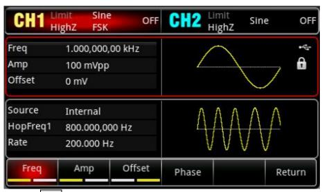
Press the softkey Freq to set the frequency, use the numerical keyboard to enter 2 and then select the unit of parameter to kHz.
