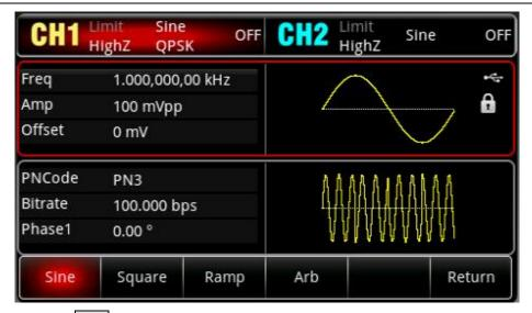
Press the softkey Freq, use the numerical keyboard to enter 2 kHz.
