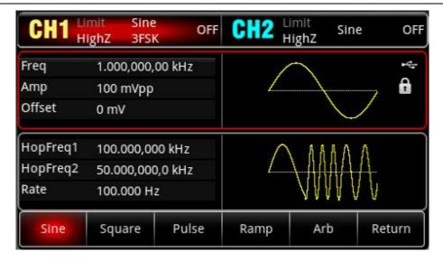
Press the softkey Freq to set the frequency, and then use the numerical keyboard to enter 2 kHz.
