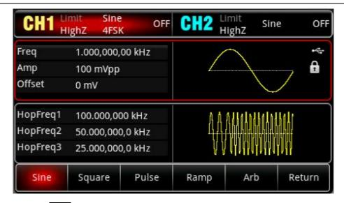
Press the softkey Freq to set the frequency, and then use the numerical keyboard to enter 500 Hz.
