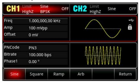
Press the softkey Freq, use the numerical keyboard to enter 2 kHz.
