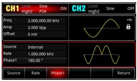
To view the modulation waveform of PSK through an oscilloscope as shown in the following figure.
