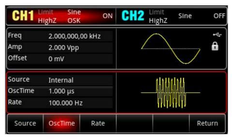
To view the modulation wave of OSK through an oscilloscope as shown in the following figure.
