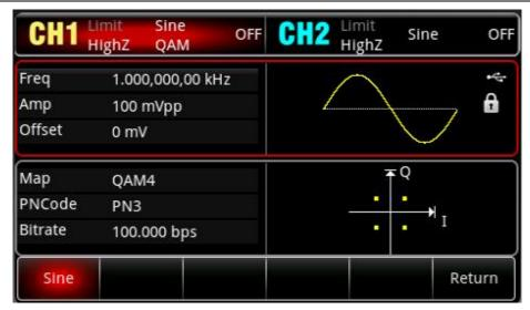
Press the softkey Freq, and then use the numerical keyboard to enter 2 kHz.
